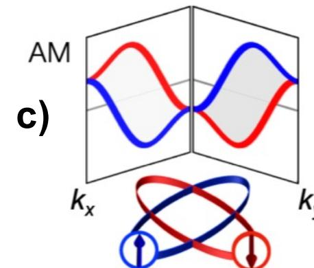
c) Spin split band structure of a model altermagnet (FM)
