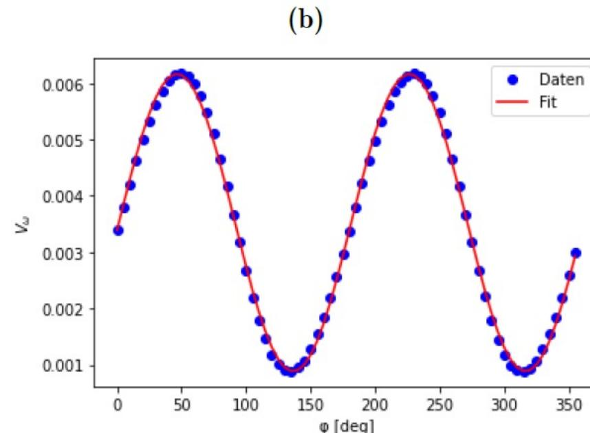
Examples of the first harmonics for a magnetic field of (a)  $\mu_0 H = 80 \text{ mT}$  and (b)  $\mu_0 H = 350 \text{ mT}$ .
