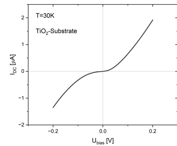
Tunneling curves show typical nonlinear behavior around  $U = 0V \rightarrow$  Tunneling seems oK.
