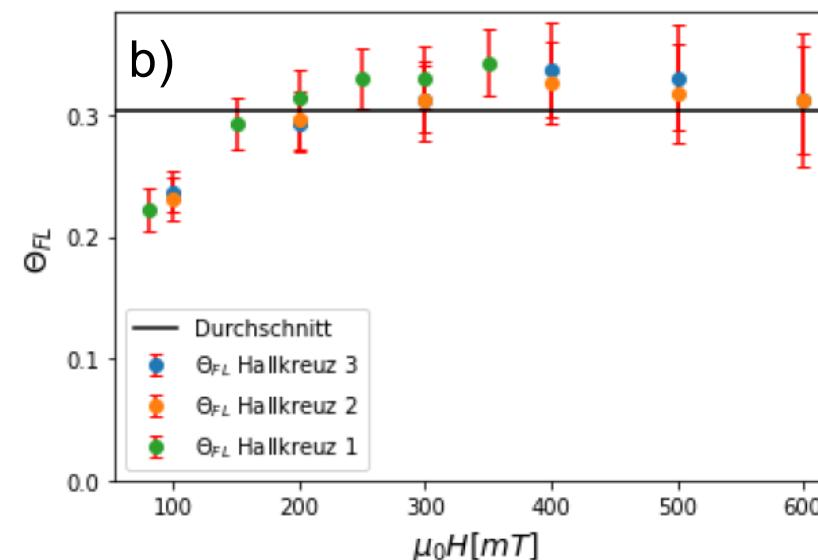
The (a) damping-like  $\theta_{SHDL}$  and (b) field-like  $\theta_{SHFL}$  SHA's of the Hall crosses at different applied fields → Torques seem to be present → Antiferromagnetism
