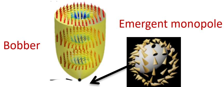
*Metastable bobbers produced by either field-cooling or field-tilting in LTEM*
