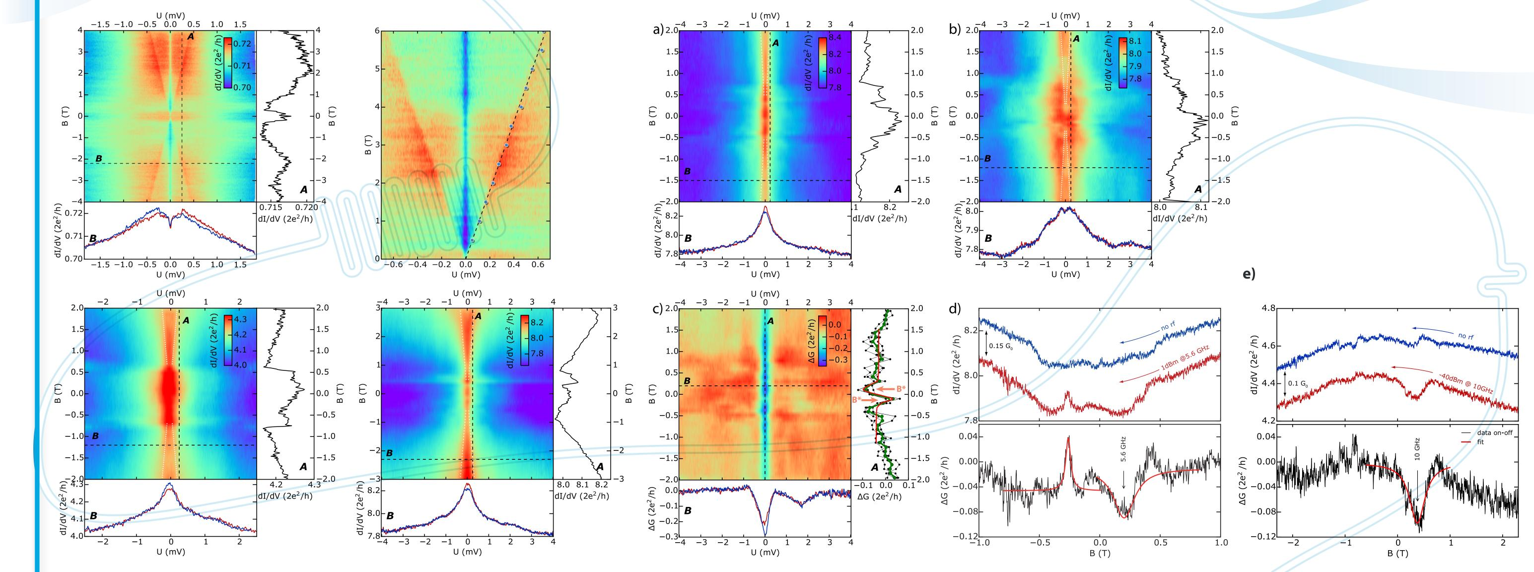
Differential conductance maps of Pd and Co/Pd hybrid point contacts as a function of bias voltage and magnetic flux show a Zeeman splitting in the LDOS. Line traces at the positions A and B indicated in the pseudocolor plots resemble the magneto-conductance and point contact spectra.
