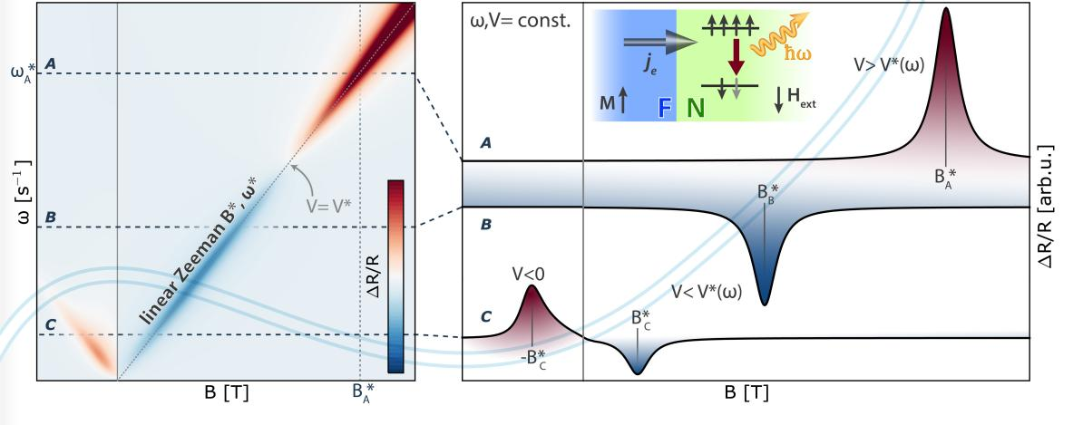
Expected transport behaviour of a diffusive F/N hetero-point contact due to spin-flip photoemission and absorption according to the semi-classical transport theory reported in:
