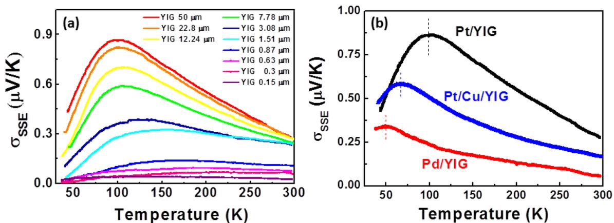
Figure 1. (a) Temperature dependent SSE coefficients ( $\sigma_{SSE}$ ) of YIG thin films with a wide range of thicknesses. (b) Temperature dependent  $\sigma_{SSE}$  measured at Pt/YIG, Pt/Cu/YIG, and Pd/YIG hybrids. The thickness of YIG films is 50  $\mu\text{m}$ .
