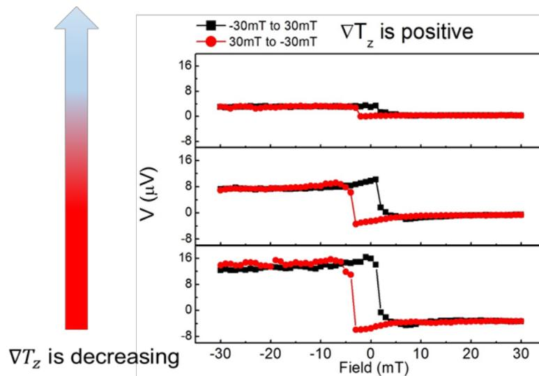
ANE on CoGd(20nm) / Si thin film with out of plane temperature gradient
